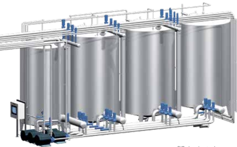
CIP cleaning tanks
